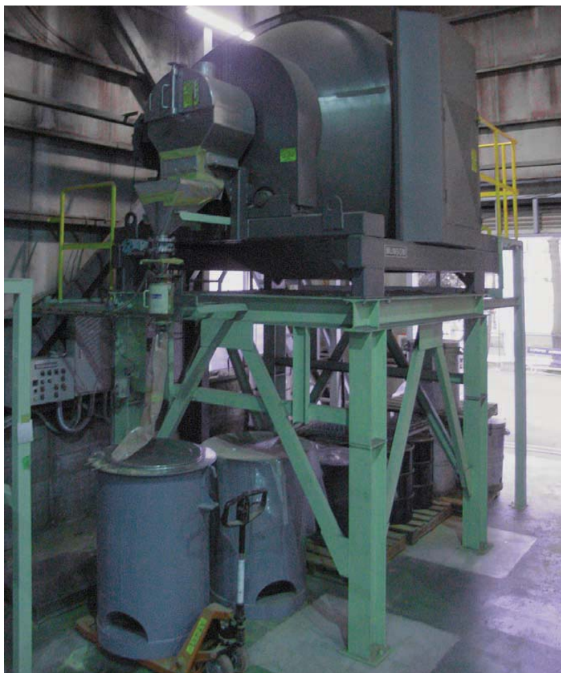
Figure 3: The 2.5 cu m capacity rotary batch mixer evacuates fully, eliminating wasted material and allowing rapid, thorough cleaning between changeovers.
