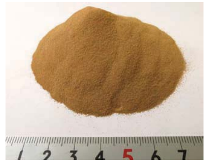
Figure 6: Nippon Atomized Metal Powders' main product for oil-less bearings is partially premixed copper-tin bronze powder.
