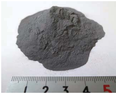
Figure 4: Copper-tin pre-alloyed bronze powder for diamond cutting is the finest (20-30 micron) homogenised in the 2.5 cu m capacity rotary batch mixer.
