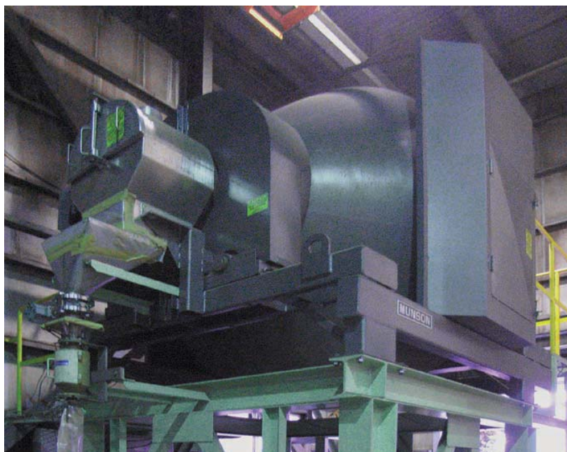
Figure 2: As the rotary batch mixer discharges, particle size distribution remains unchanged, which was not the case with other mixers used by Nippon Atomized Metal Powders.
