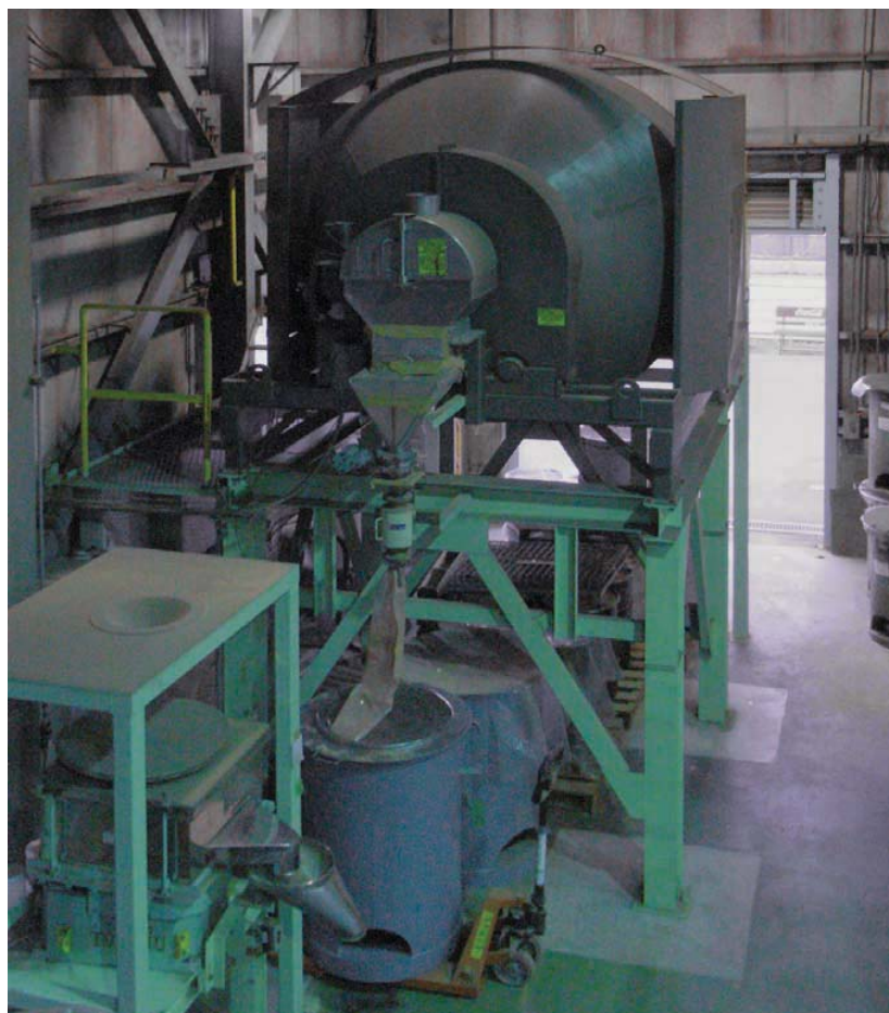
Figure 1: Batches of metal powder typically weighing 4,000–5,000 kg are loaded into the Munson rotary batch mixer from an overhead container that is moved into position by a crane.
