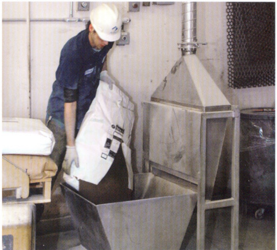
Operator dumps "hand-adds" into mixer from floor above.
