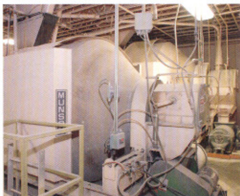
The rotary batch mixers discharge with little or no product residual, simplifying changeovers.
