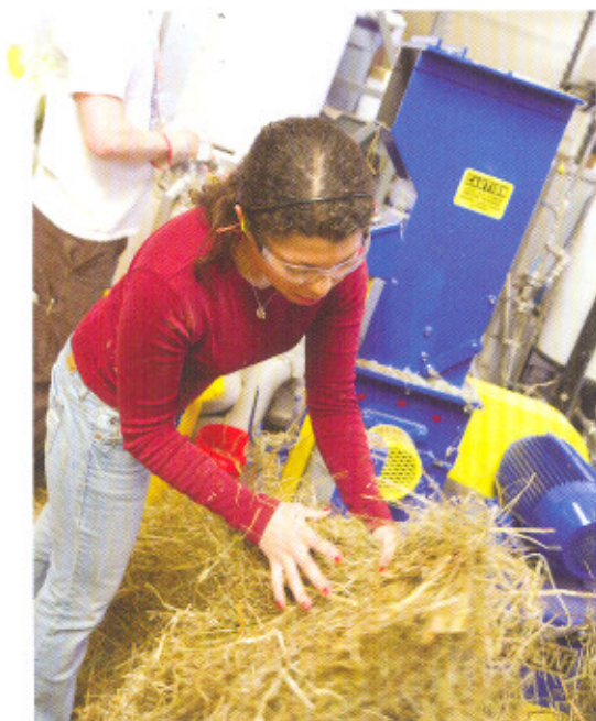
Screen classifying cutter downsizes raw materials into uniform particles at University of Maine's Process Development Center. In one alternative energy project, perennial grasses and hay are pelletised to make compressed biofuel pellets.
