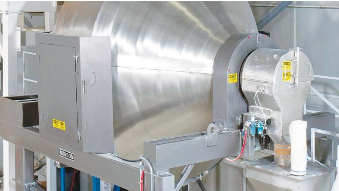
Upon discharge, the 140-cu. ft.-capacity rotary batch mixer evacuates completely with little or no residual, allowing fast, thorough cleaning between batches. Continuous rotation of the drum assures that all materials remain in motion, preventing segregation in batches of varying material densities.
