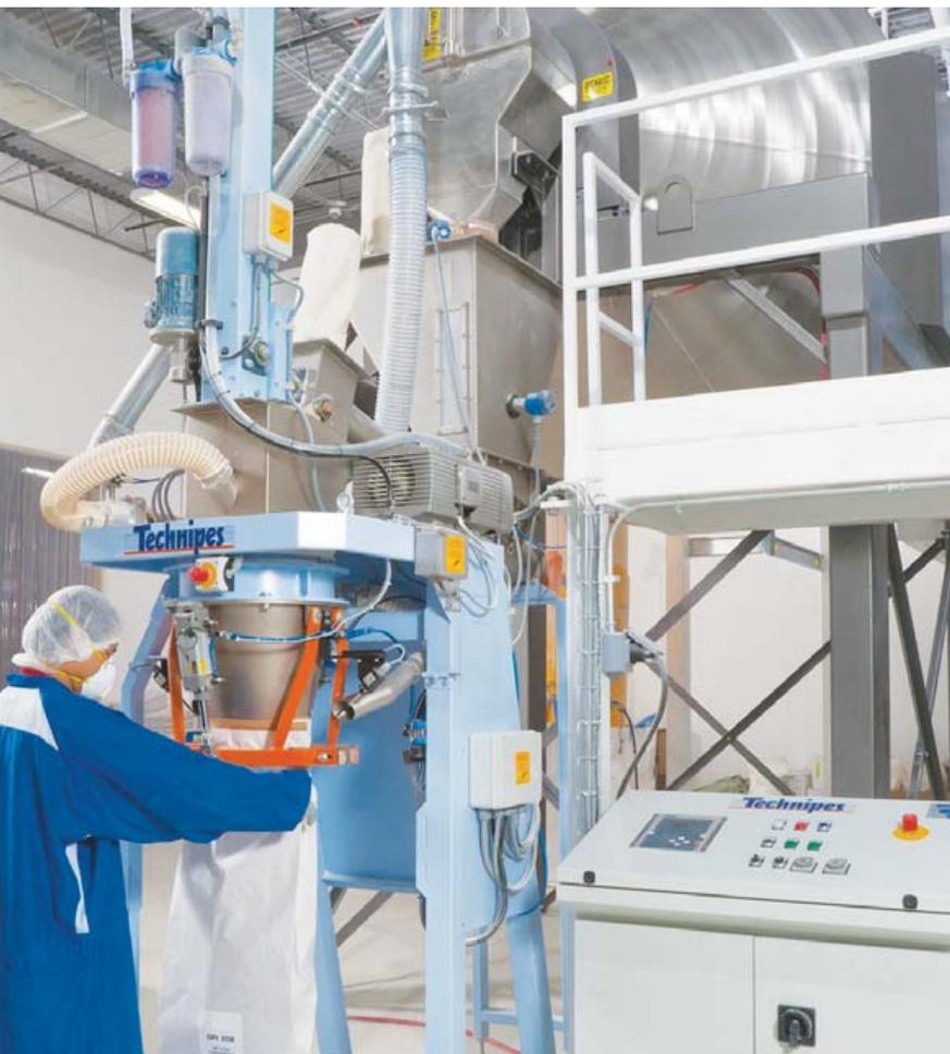
**Powders discharge from mixer into hopper and then to bagging machine, which fills 55-lb. bags or 2,000-lb. bulk bags.**
