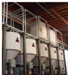
Biosphere Industries, a manufacturer of biodegradable packaging and biodegradable bakeware, needed a highly accurate ingredient batching system to help meet its sustainability goals. The company interviewed several candidate vendors and, on the basis of speed, repeatability, lead time for completion and cost, selected a turnkey automated batching system. **To read about this success story, turn to page 20.**
