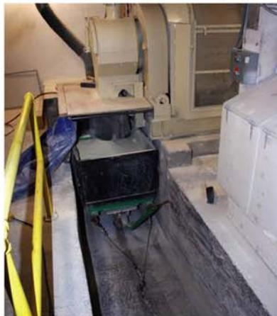
The batch is rapidly discharged from the mixer into a cart that transports it to the furnace.
