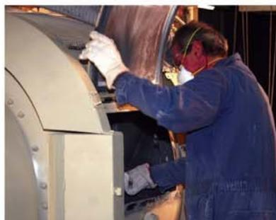
Access doors facilitate interior inspection, cleaning and maintenance.
