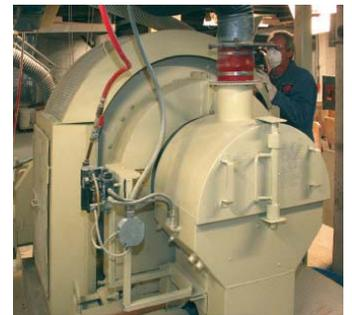
Kopp replaced a rotary pan mixer with a Munson rotary batch mixer — a horizontal, rotating drum with a stationary inlet at one end and a stationary outlet at the other. Mixing flights, or baffles, tumble the batch in a multi-directional manner.
