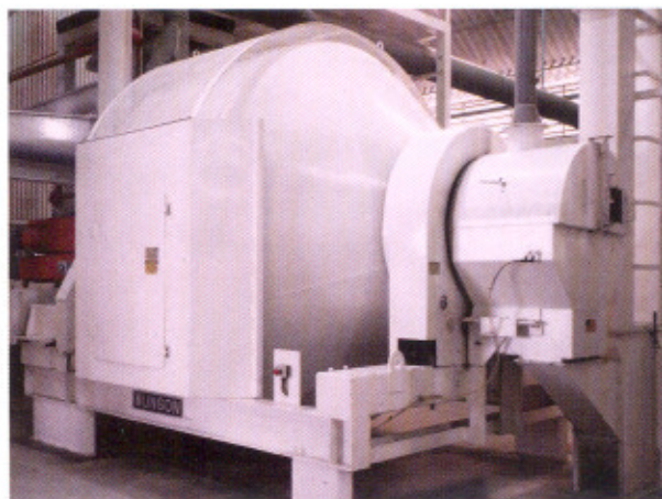
The rotary mixer evenly impregnates microgranules with liquid chemicals to produce insecticides
