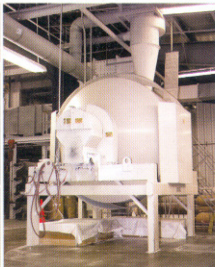
Munson says its 700-TSC-300 achieves batch uniformity in about three minutes and discharges with no residue.
