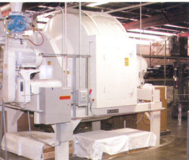
Rotary batch mixer controls particle-size distribution.
