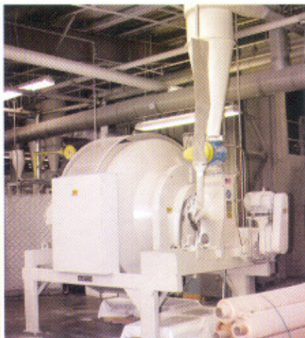
Munson says the mixing action of this rotary batch mixer provides homogenous, high quality recycle.
