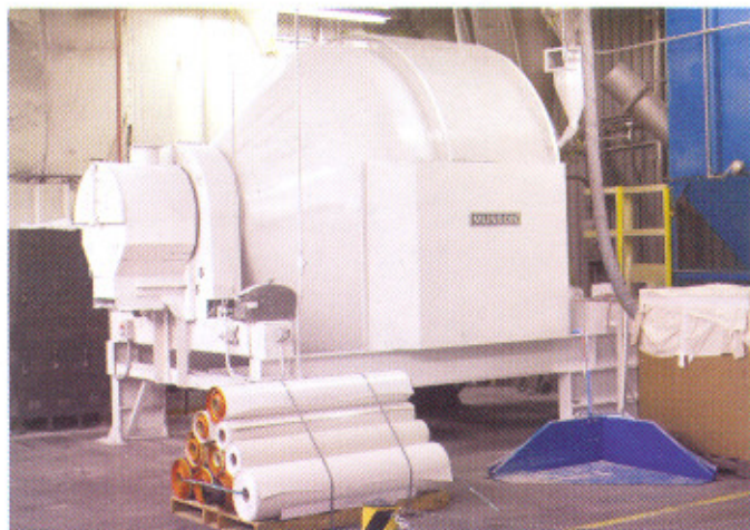
Omnova invested in a second, smaller rotary batch mixer to meet growing in-house demand for recycled material.
