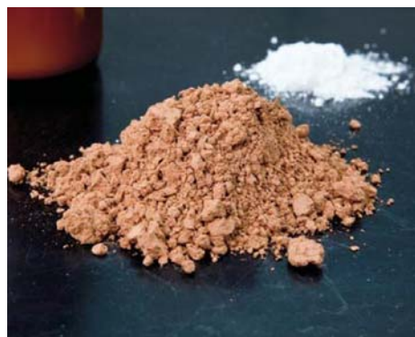
Iron oxide (foreground) and titanium dioxide are basic raw materials for CEI's face powders
