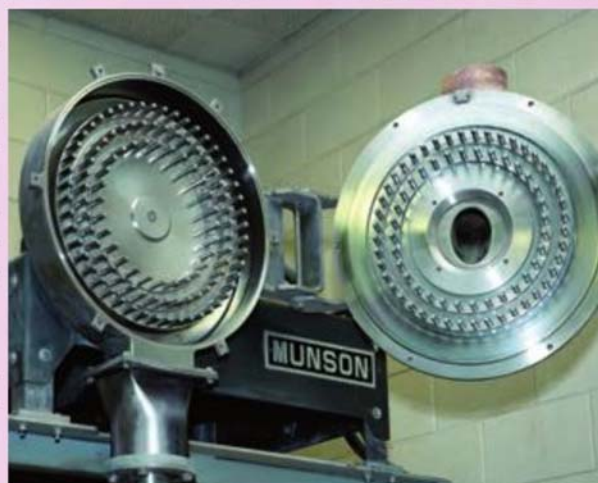
Access to the interior of the pin mill is achieved by simply unlatching the cover
