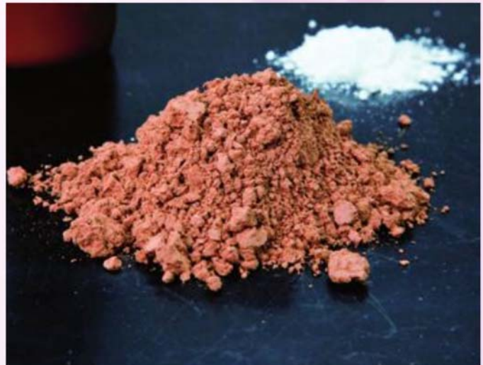
Iron oxide (foreground) and titanium dioxide are basic raw materials for CEI's face powders
