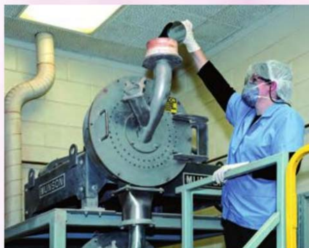
An operator adjusts the inlet to the pin mill
