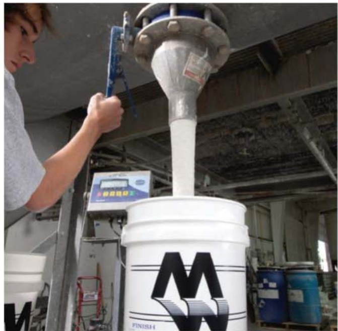
Heavy duty blended topcoats, typically comprising 75% solids, are discharged into 5-gal pails.
