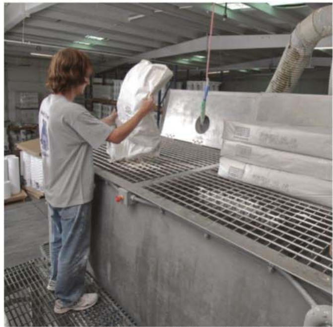
Bags of pigments and fillers are added through the blender's safety grate.
