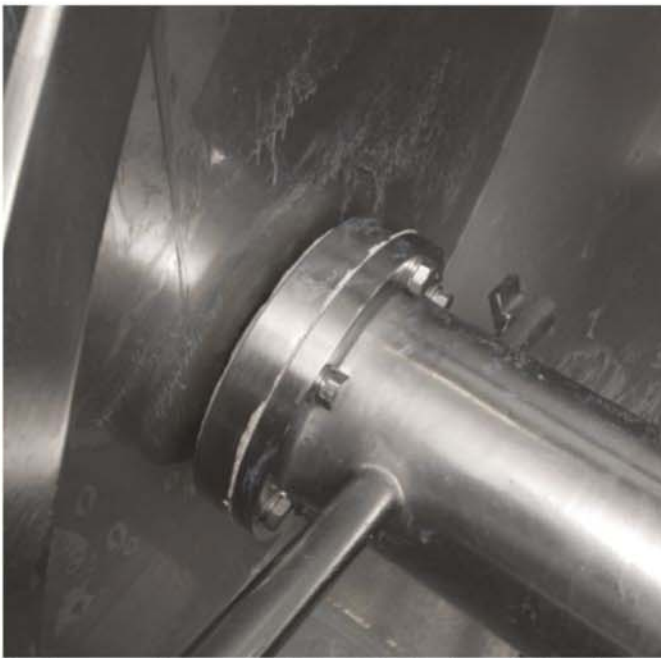
An air purge seal between the shaft and the blender wall drives abrasive particles away from the seal, preventing premature wear and leakage.
