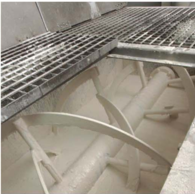
The tight clearance between the ribbon blades and blender trough minimizes residual material after discharge.
