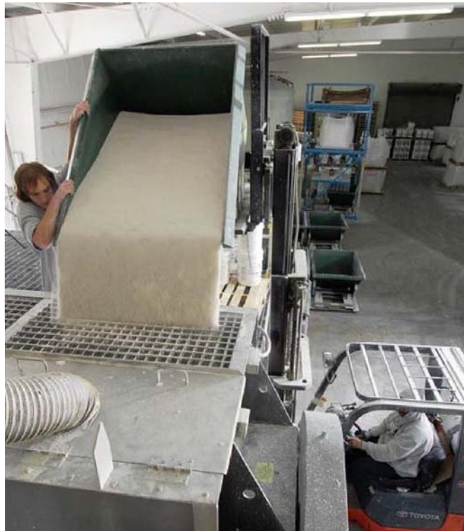
ABOVE: Operator adds pre-weighed aggregates from self-dumping hopper to the Munson HD-48-SS ribbon blender
