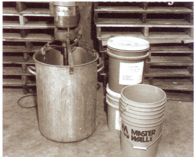
Master Wall's original two-speed propeller-type blade mixer produced only three 19-litre pails of stucco per batch.
