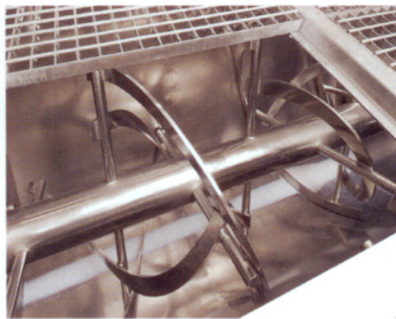
At the top of the 2839-litre capacity ribbon blender, negative-pressure dust collectors pull dust into a bag house as the blender fills 19-litre pails of exterior coatings products.
