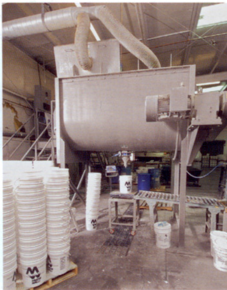
At the top of the 2839-litre capacity ribbon blender, negative-pressure dust collectors pull dust into a bag house as the blender fills 19-litre pails of exterior coatings products.
