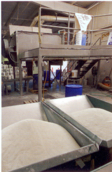
Heavy, abrasive aggregates (foreground) will be added from self-dumping hoppers to the Munson HD-48-SS ribbon blender (background).
