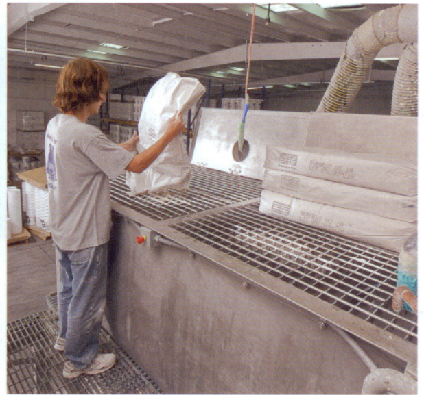
23kg bags of pigments and fillers are added through the blender's safety grate.
