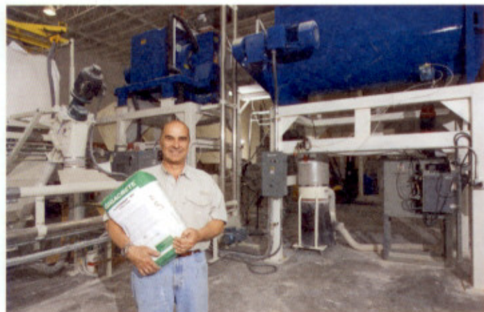
ABOVE: Andrew Dennis, chairman and founder of GigaCrete, displays bag of PlasterMax ICF building product. Behind are Munson rotary batch mixer (L) and continuous paddle blender (R)
