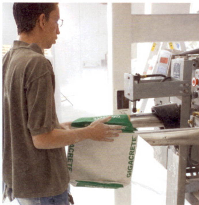
ABOVE: Operator fills bag from turbopacker below the rotary batch mixer
