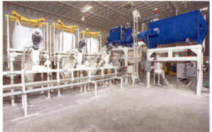
ABOVE: Powder transfer system, consisting of five bulk bag dischargers, prepare a batch as aeromechanical conveyors transport material to one of the two mixers.
