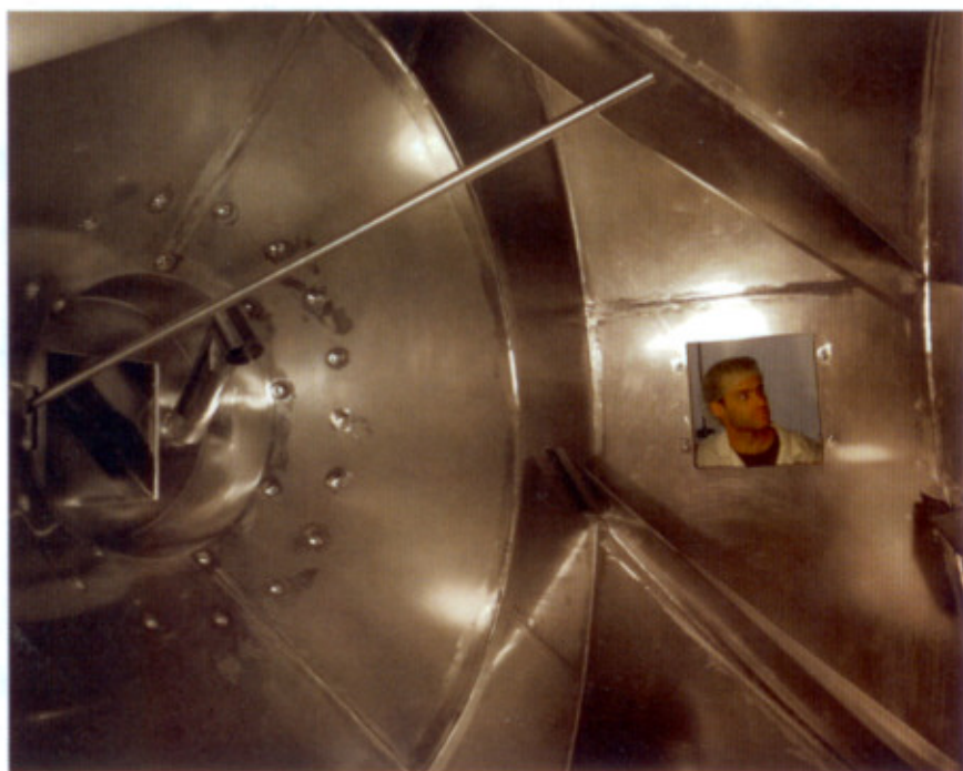
Pro-X Nutraceuticals installed a mixer that includes a rotating drum with internal mixing flights. It achieves batch uniformity in less than 3 minutes.
