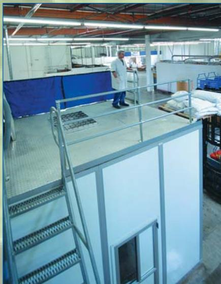
*Figure 1 – Bags of raw material forklifted to mezzanine level are manually dumped through a screen (left of operator) into a rotary batch mixer located in the room below, in compliance with US FDA's Good Manufacturing Practices*
