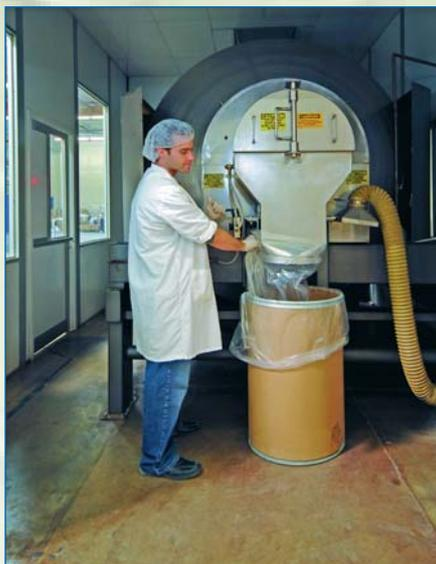
*Figure 3 – Internal mixing flights elevate the material which is discharged through a plug gate valve into plastic-lined drums*
