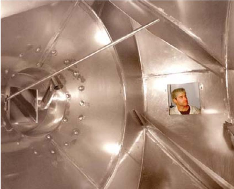
Rotating drum with proprietary mixing flights achieves total batch uniformity in less than three minutes.
