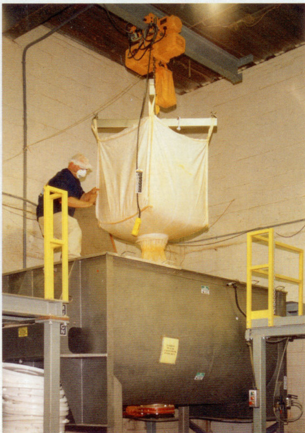
Most of the spice ingredients are received in 50-lb bags or boxes, but some, such as salt, come in bulk bags that are emptied into the paddle mixer by means of a hoist.
