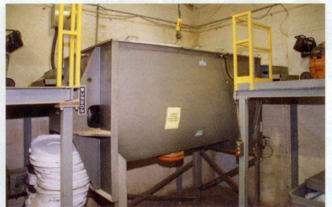
This 150-cu-ft paddle blender mixes most of the spices produced by J.O. Spice Co.
