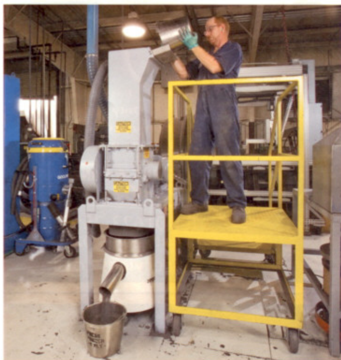
ABOVE: Operator batch feeds scrap into the cutter and removes downsized material
