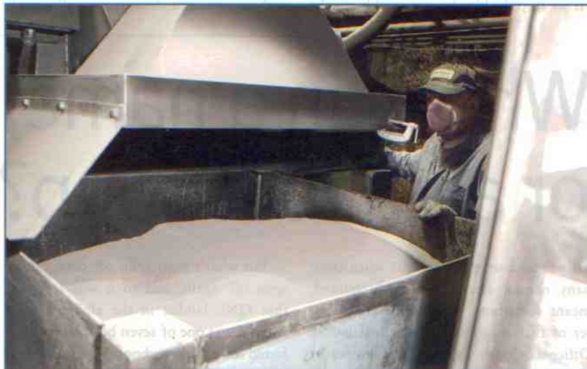
Figure 3. Once blended, the load is discharged to the hopper for onward transport to packing and dispatch areas.
