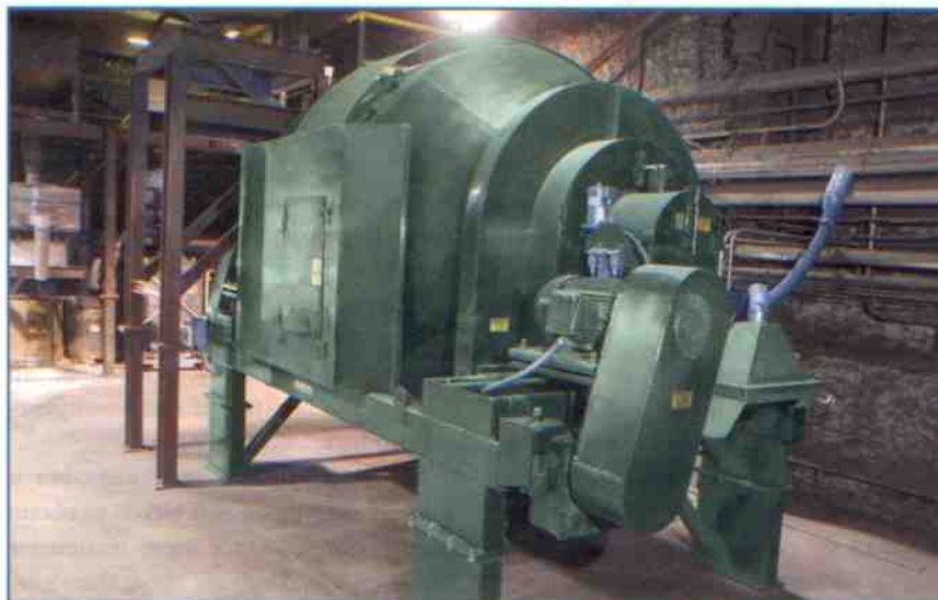
Figure 2. Relatively compact in itself, the blender can handle batch load from 2000 kg to 20000 kg with equal efficiency.
