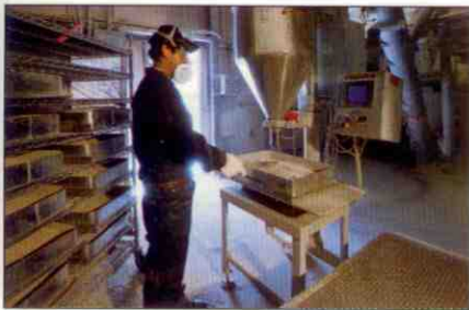
Charging tray is filled with blend.
