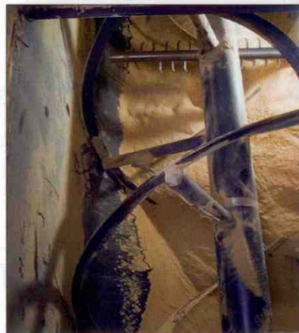
Ribbon blender blades produce counter-directional flow to blend materials.
