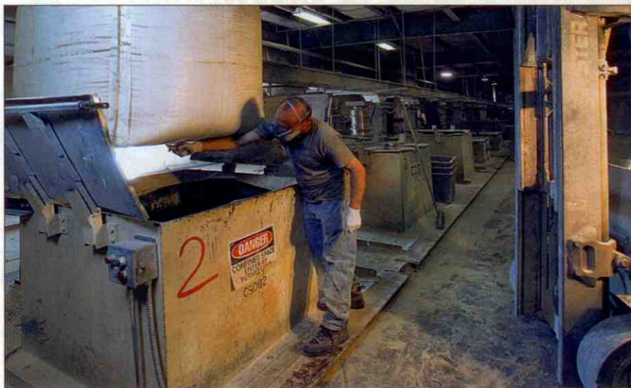
From bulk bag, operator loads one of 12 ribbon blenders with wood flour or resin.
