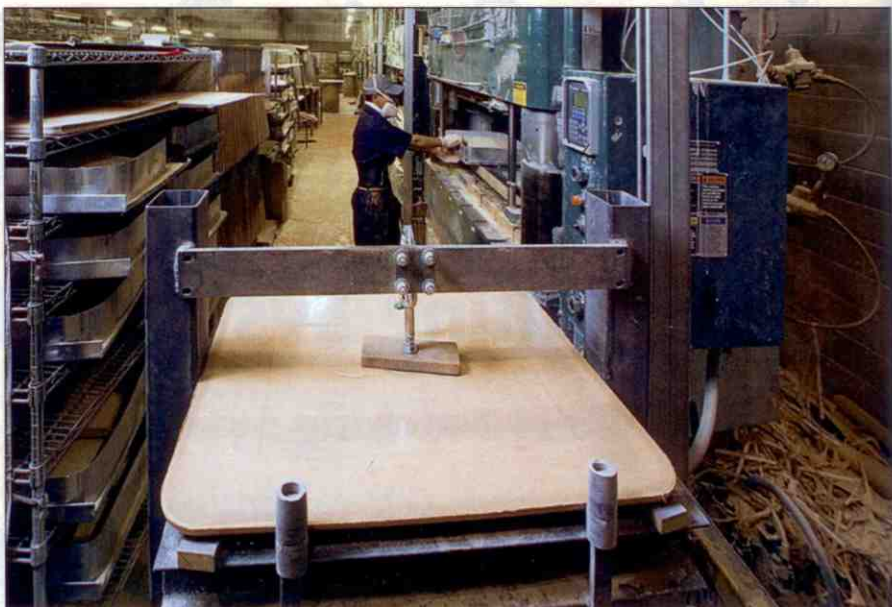
Operator loads charges into hydraulic press which molds furniture components.
