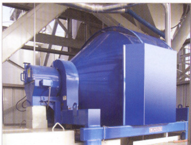
A 2.6 m 3 Munson 700-TH-90-AR rotary batch mixer gently yet efficiently blends dry cement mixes in less than 3 minutes with 100% uniformity. Gentle mixing preserves the texture of the coarse material, which is necessary to maximise the strength of the cured product.
