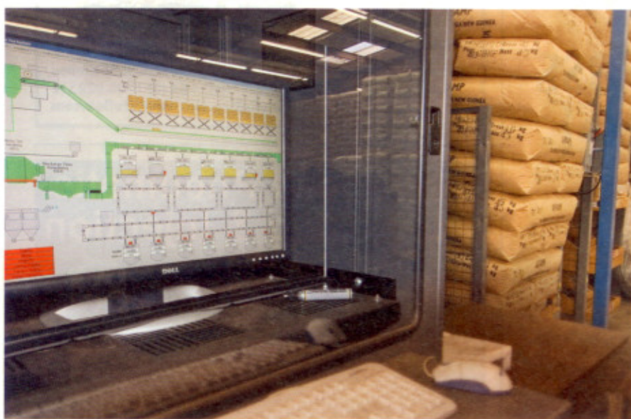
From this station, a technician controls the proportions for each batch of tea produced
