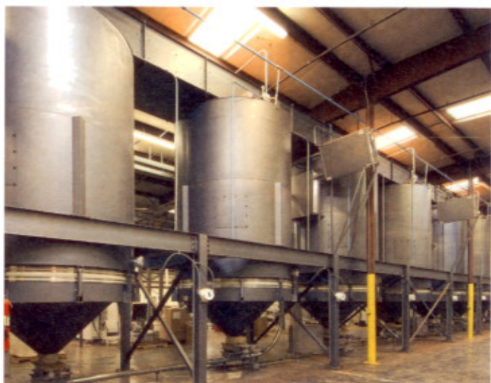
ABOVE: Each storage vessel holds a specific type of tea that will be used in a blend produced by S&D Coffee
