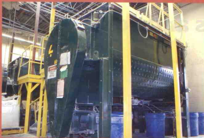
Bottom-mounted gearboxes and drives (behind the front protective cover) consume 1.1 m 3 less floor space than side-mounted versions.
