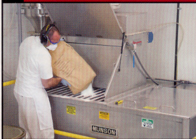
Figure 3. Solids are fed to the mixer with hood cover and exhaust fan for containment.
