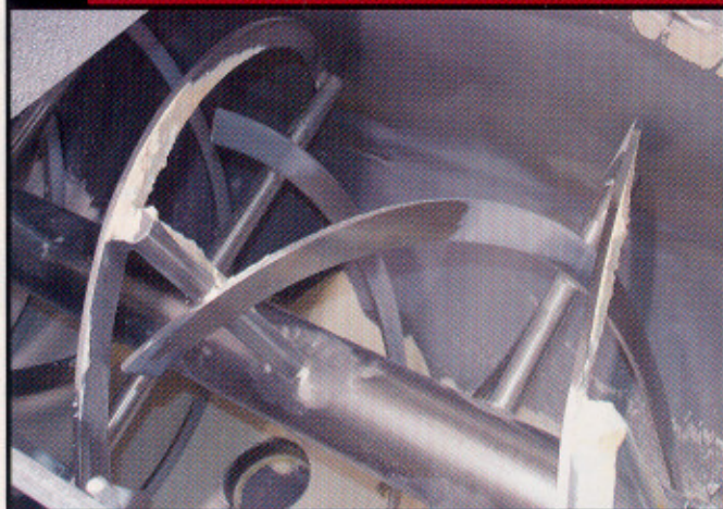
Figure 2. Blades of mixer move in opposite directions, promoting solid blending.
