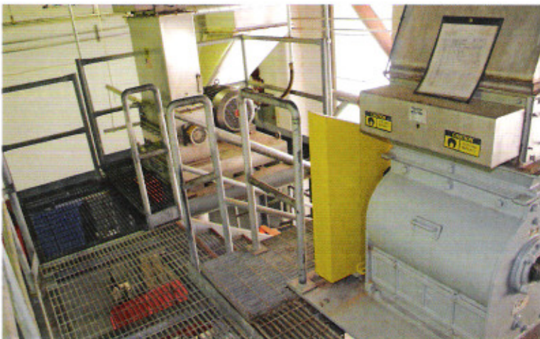
ABOVE: ginger root, cassia bark and cola nuts are conveyed by rigid auger through a magnet and into the Munson knife cutter.
