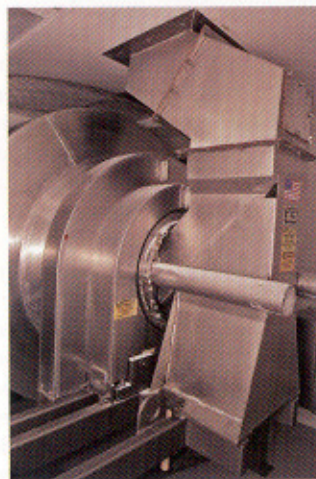
A Munson rotary mixer operated by Nutri-Force Nutrition creates uniform blends in 3 minutes, about 10 times faster than other mixers.
