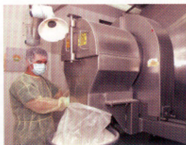
The mixer completely evacuates material from the mixing drum between runs, expediting the sanitizing process for Nutri-Force, an FDA-licensed facility.
