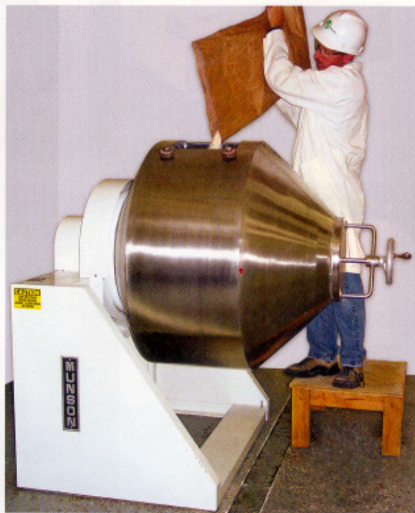
ABOVE: United-Tech blends 227 kg every 3-5 minutes. By unloading quickly, the blender maximises the number of batches United-Tech is able to blend. Evenly spaced baffles inside the rotating drum set powdered ingredients in motion with a gentle cascading action.
