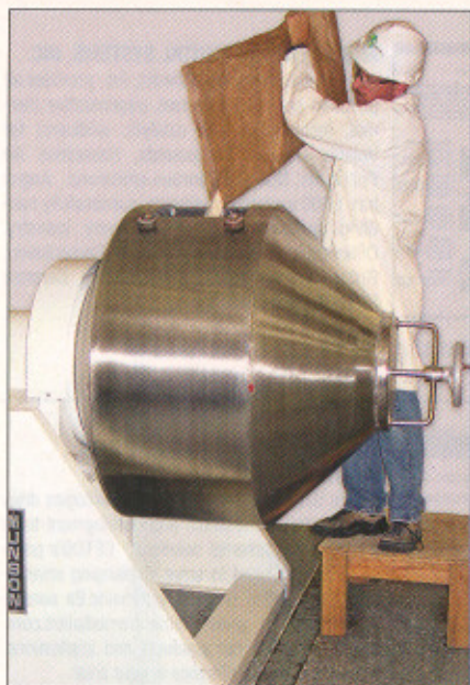
United-Tech blends 500 lb. every 3 to 5 minutes. By unloading quickly, the blender maximizes the number of batches they are able to blend. Evenly spaced baffles inside the rotating drum set powdered ingredients in motion with a gentle cascading action.
