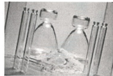
Examples of some finished goods—syringe cartridges and vials—along with the raw material from which they are made.
