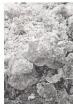
Recycled cullet is an important component of Kimble's pharmaceutical glass recipes. The cullet
