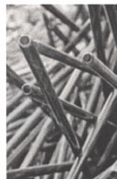
Recycled cullet includes material rejected from the manufacturing process. Some examples are the rejected amber and clear (flint) tubing shown here.
