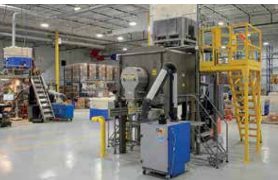
One receiving hopper containing a blended batch is rolled away from the mixer (foreground) as another fills a packaging machine surge hopper (rear left).
