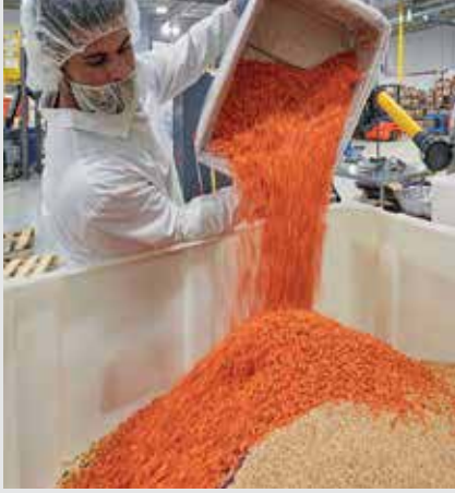
Ingredients are emptied into a 0.56 m 3 (20 cu ft) hopper that is forklifted into position above the mixer's inlet.
