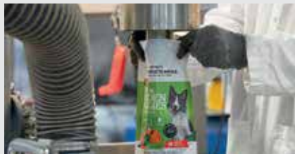
Pouches of Dr. Harvey's product—a blend of 15 to 30 dry ingredients—are filled at the packaging machine.
