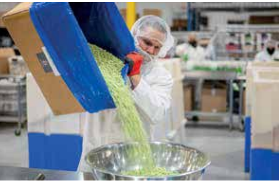
Operators weigh and empty ingredients into bowls which are emptied into a 0.56 m 3 (20 cu ft) hopper that feeds the Rotary Batch Mixer.
