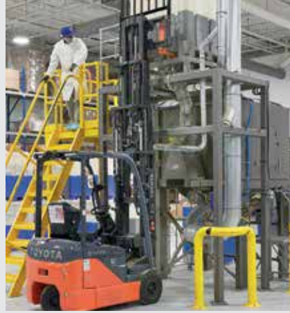
Batched ingredients gravity discharge from the 0.56 m 3 (20 cu ft) hopper into the Rotary Batch Mixer of equal capacity.
