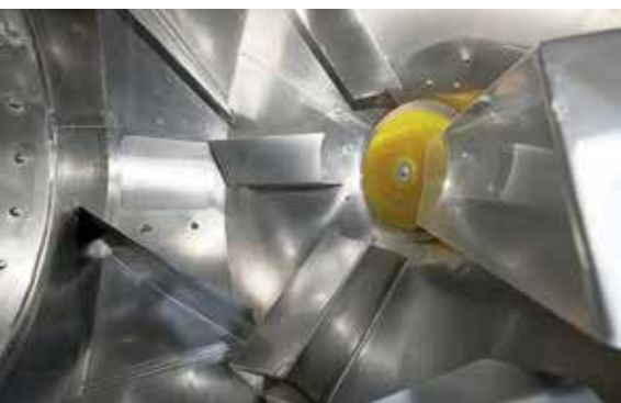
Proprietary mixing flights impart a tumble-turn-cut-fold mixing action that causes particles to recombine 288 times per minute, yielding uniform blends in about five minutes.
