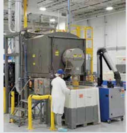
Blended ingredients are transferred from a receiving hopper below the mixer's plug gate discharge valve, into the packaging machine inlet.
