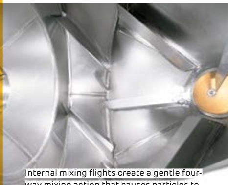
Blends discharge with no residual through the stationary outlet into bulk bags that are transferred to the packaging lines.
