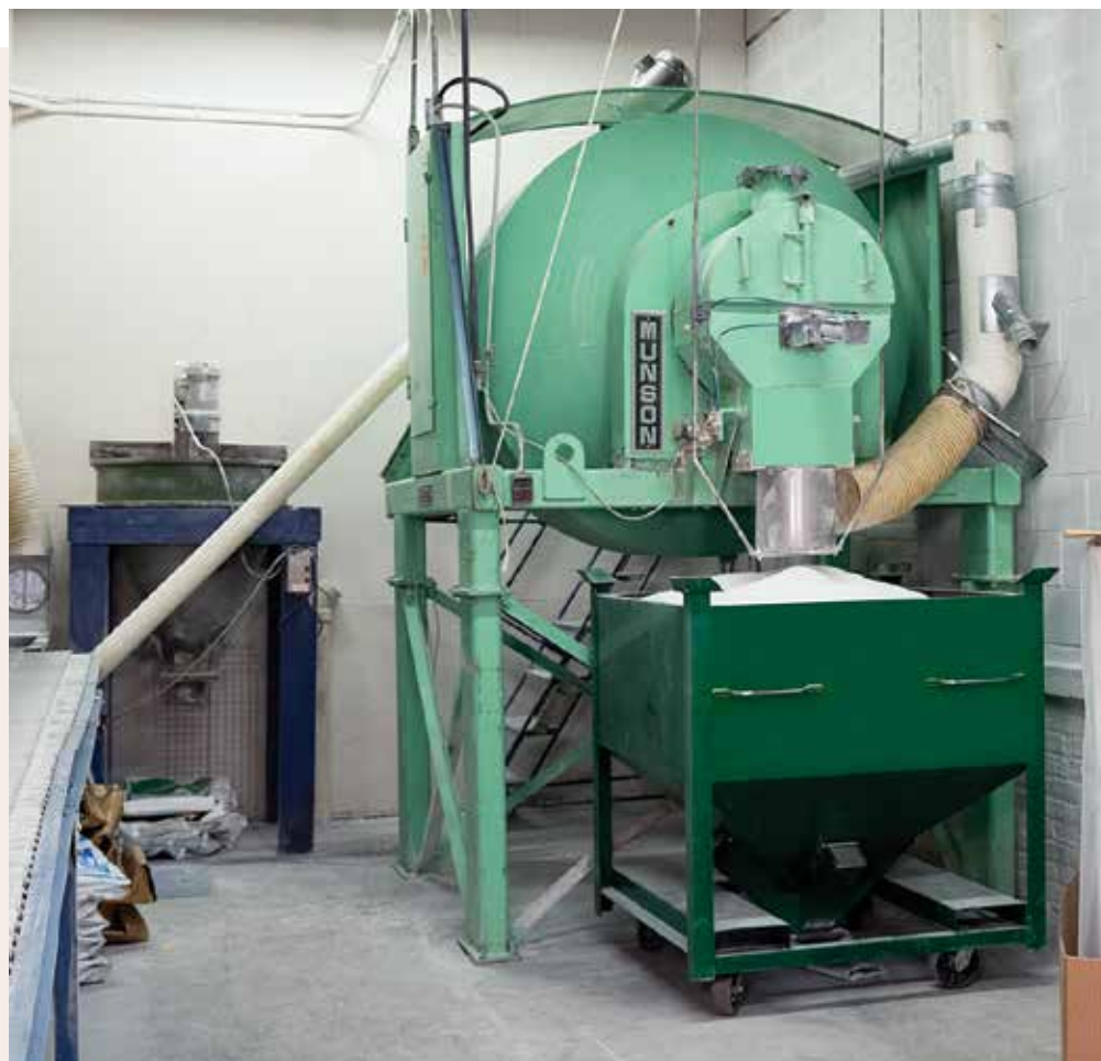
IN THE MIXING ROOM a rotary batch mixer distributes resins, waxes and fillers uniformly in 1,000 lb. batches. Courtesy Munson Machinery
