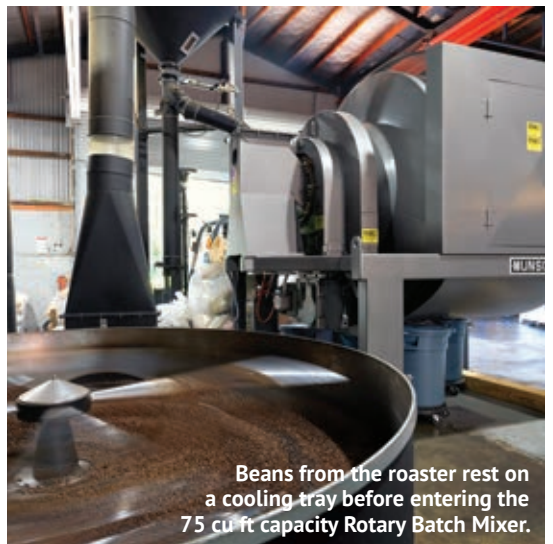
The 700-TS-75-MS Rotary Batch Mixer has a gentle four-way mixing action that eliminates or minimises breakage of the beans.
