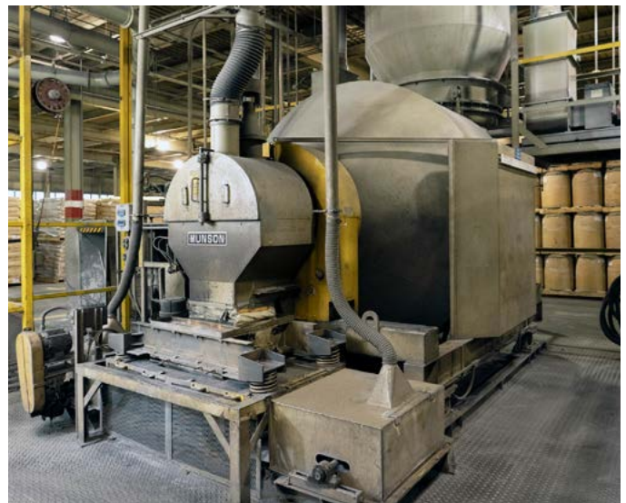
One of two Munson Rotary Batch Mixers, model 700-TSC-180-MS, that have been in operation at Plastics Engineering Co. since 1983. All photos courtesy of Munson Machinery Co.
