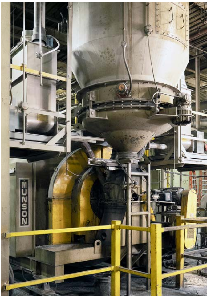
To fill the vessels, a pneumatic conveyor transports resins from compounding lines to a holding hopper. (Left) Continuous rotation of the drum during discharge prevents stratification of ingredients having disparate sizes, shapes and bulk densities, and empties the batch in a steady stream. (Top-Right) Hinged access doors at either side of the vessel provide access to all material contact surfaces for cleaning and visual inspection. (Bottom-Right)
