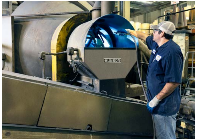
To fill the vessels, a pneumatic conveyor transports resins from compounding lines to a holding hopper. (Left) Continuous rotation of the drum during discharge prevents stratification of ingredients having disparate sizes, shapes and bulk densities, and empties the batch in a steady stream. (Top-Right) Hinged access doors at either side of the vessel provide access to all material contact surfaces for cleaning and visual inspection. (Bottom-Right)
