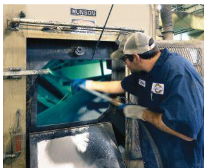
The hinged access doors at either side of the vessel provide access to all material contact surfaces for cleaning and visual inspection.
