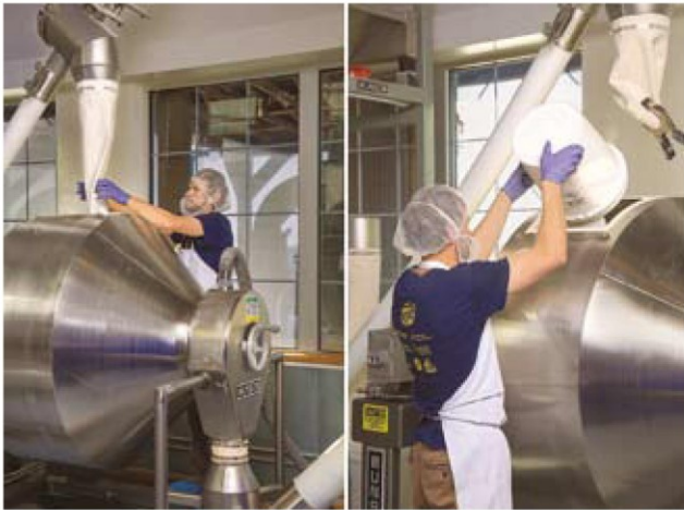
The mixer can be loaded with 227 to 317 kg of material in five minutes, with an additional minute to add secondary ingredients.
