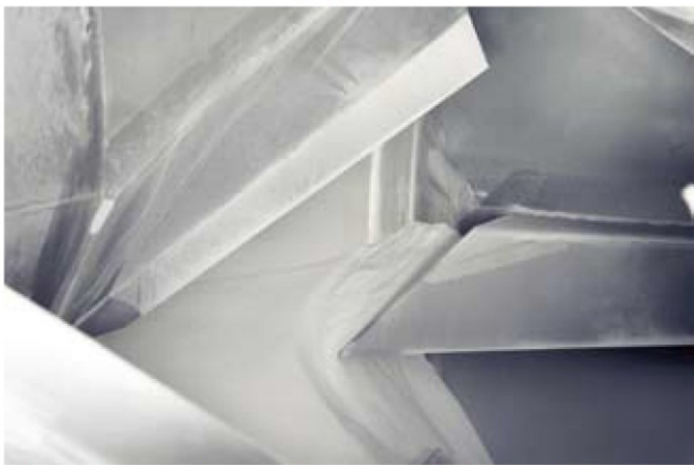
Mixing flights impart a 4-way tumble, turn, cut and fold action achieving batch uniformity in 2-3 minutes.
