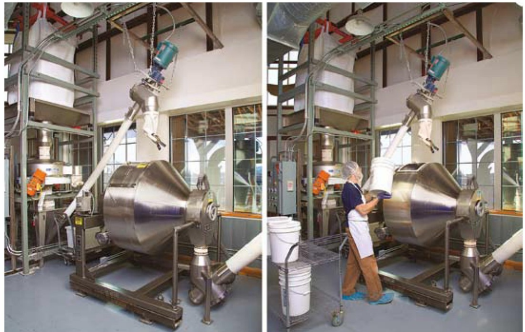
The MX-15-SS Rotary Batch Mini Mixer features a 425 l drum rotating on twin roller bearing assemblies.
