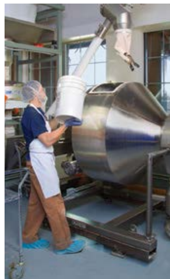
The MX-15-SS Rotary Batch Mini Mixer features a 425 l drum rotating on twin roller bearing assemblies.
