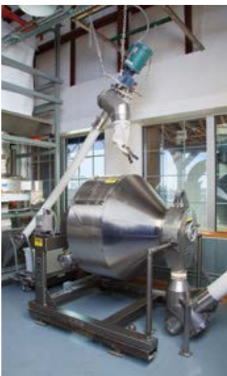
The MX-15-SS Rotary Batch Mini Mixer features a 425 l drum rotating on twin roller bearing assemblies.
