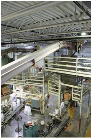
A drag chain conveyor moves batches of dry feed to the fluid bed mixer (on platform).
