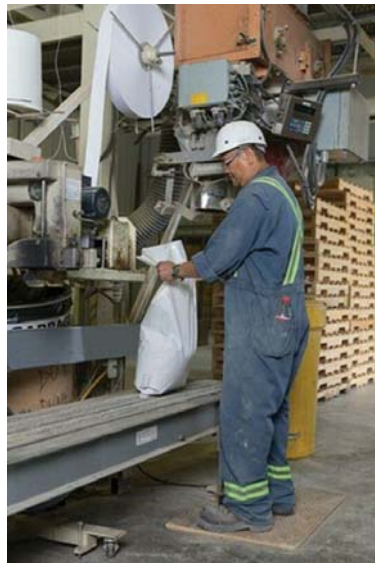
Operator fills 44-pound plastic fiber sacks at the bagging machine below the mixer and hopper
