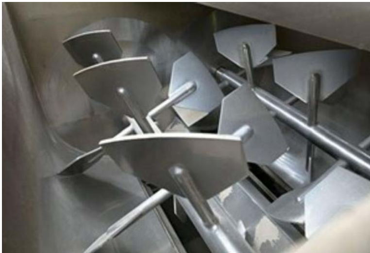
Twin paddle agitators counter-rotating within two 'U' shaped troughs create a fluidizing zone in which airborne materials intersperse rapidly with minimal degradation.
