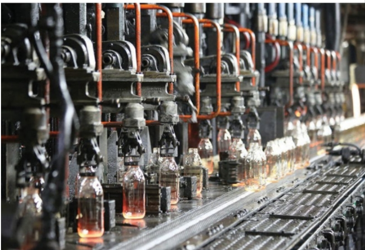
From the furnace, sodium-silicate glass is filled into molds to make clear bottles and jars.
