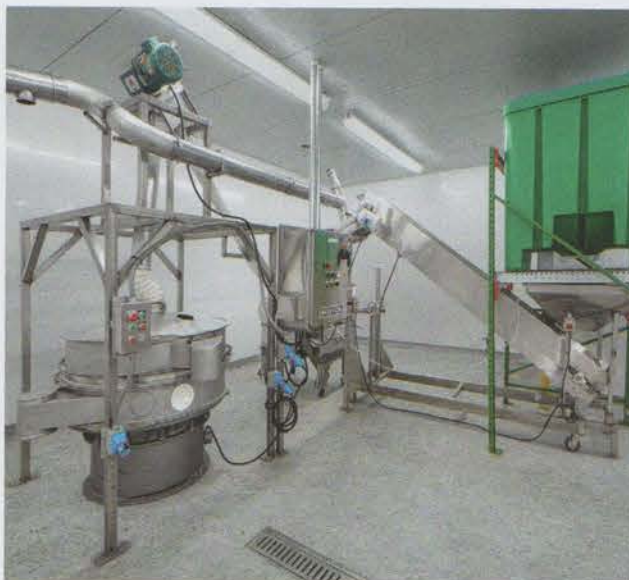
The Jewel Date Company air-dries its dates and then conveys the hardened dates to the Munson screen classifying cutter for size reduction. Photo courtesy of Munson Machinery Company, Inc.
