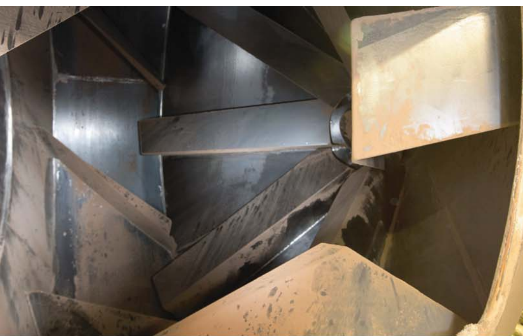
← Mixing flights lift, cut, fold and tumble the material achieving blend uniformity in one to three minutes.
