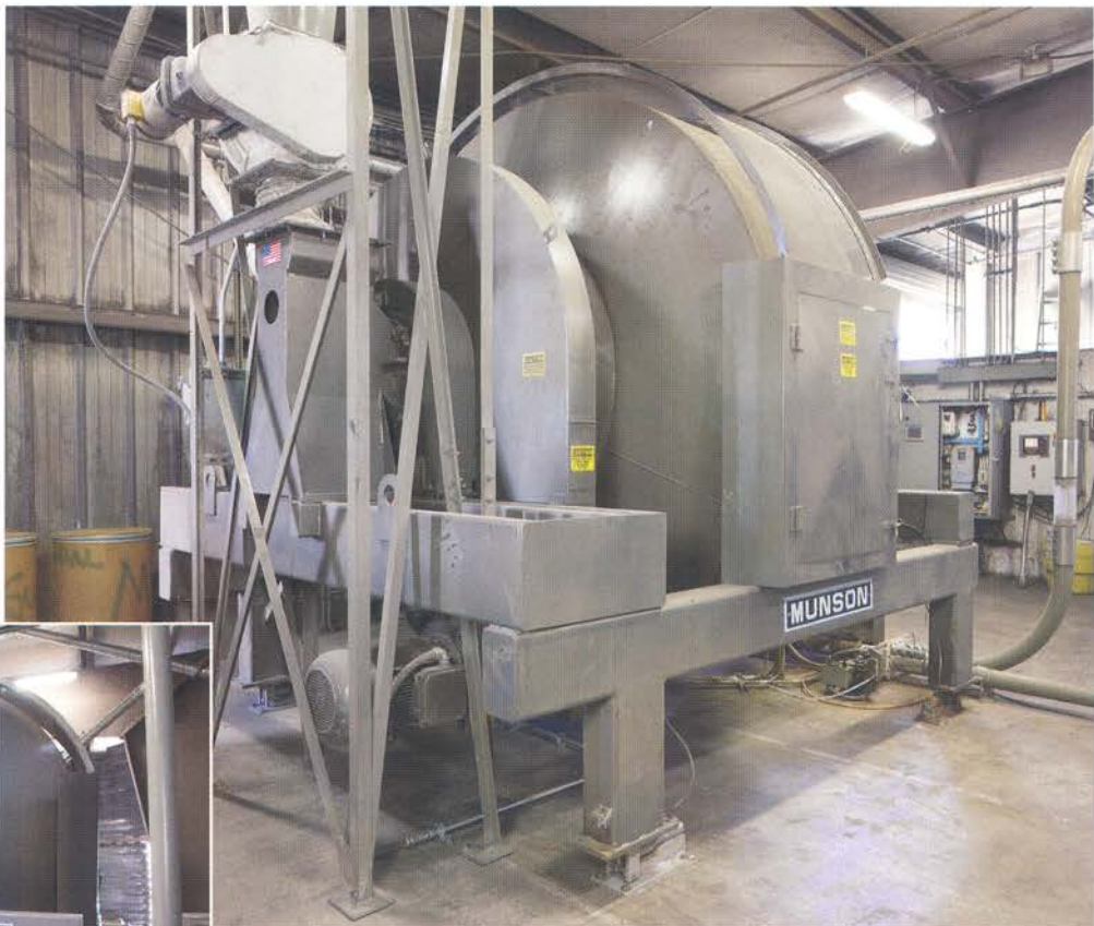
Mixer inlet (foreground) receives material from feed hoppers above.
