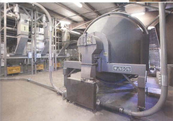
From the mixer discharge the blend is pneumatically transferred to the bag filling equipment.
