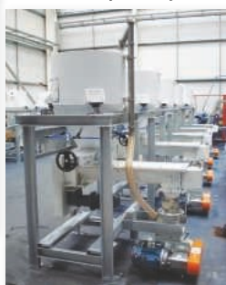
Lime Silo and Dosing System with Multiple Loss in Weight conveyors as part of an energy from waste Flue Gas Treatment Plant in Singapore.
