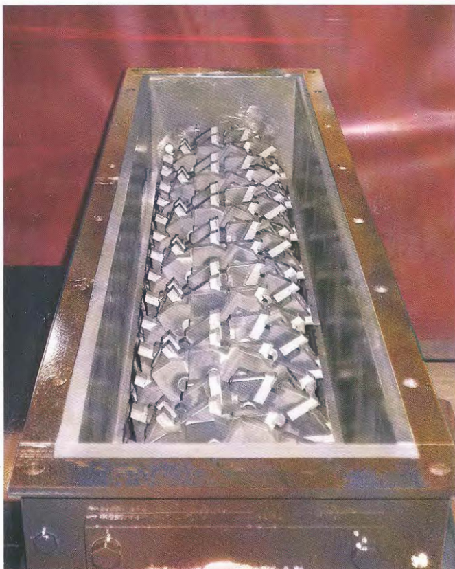
Left: The SCC Cutter's helical rotor design provides maximum throughput with minimal fines and little to no heat generation, while ensuring uniform wear.
