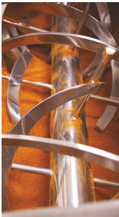
Operator weighs, measures, and loads individual spices into the Munson HD-2-1/2-5-SS Horizontal Ribbon Blender to create one of Al Dentes' many custom seasoning blends.
