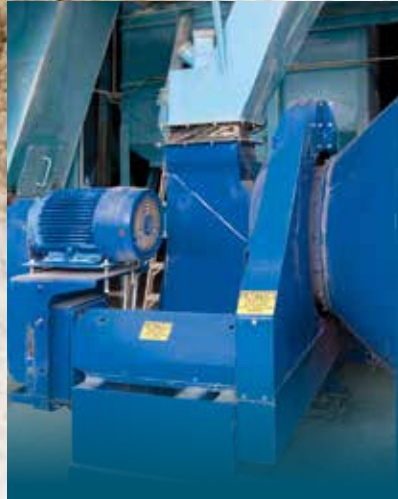
A 15 kw motor is sufficient to tumble 1361 kg batches in Rotary Batch Mixer, whereas a 37 kw motor was required to drive agitators through 453 kg batches in the company's Ribbon Blender.
