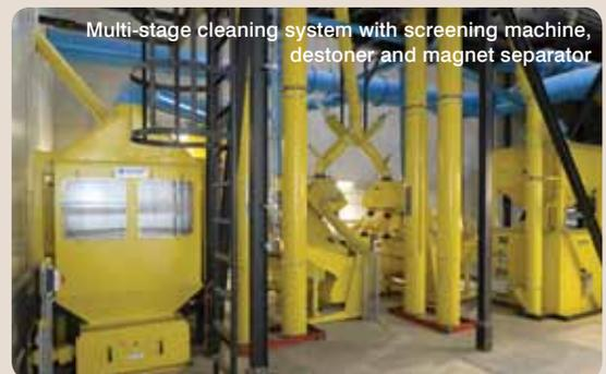
Multi-stage cleaning system with screening machine, destoner and magnet separator
