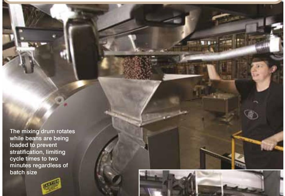
The mixing drum rotates while beans are being loaded to prevent stratification, limiting cycle times to two minutes regardless of batch size
