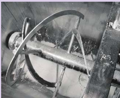
The 2:1 length-to-diameter ratio design of the double helical ribbon agitator assures thorough mixing over a range of material proportions.
