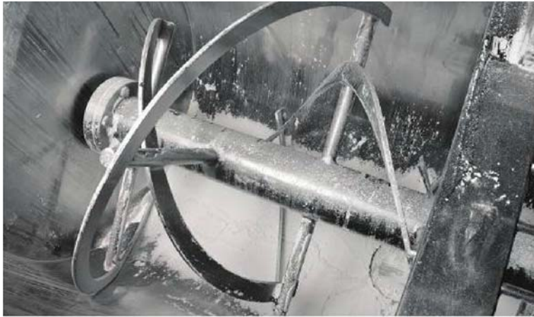
The design of the double helical ribbon agitator assures thorough mixing over a range of material properties
