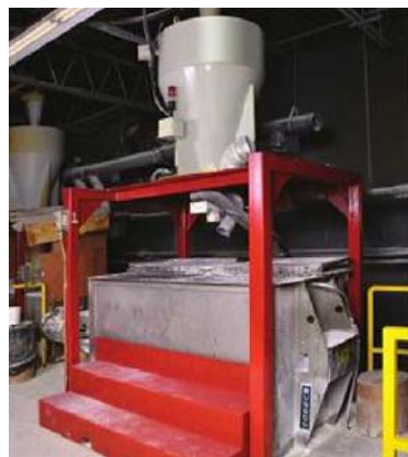
The hopper pre-weighs and adds two major ingredients to the Munson HD-36 ribbon blender
