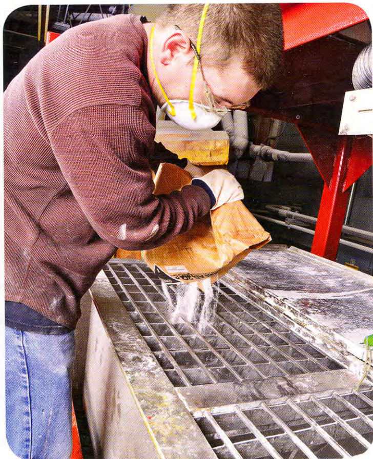
From silos located outside, the large hopper pre-weighs and adds two major ingredients to the Munson HD-36 ribbon blender. Minor ingredients are manually dumped from bags.
