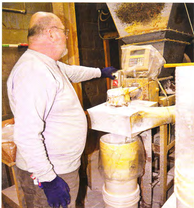
The operator fills and check weighs a 5-gal pail that will hold 50 lb of finished product. The hopper in background holds 2500 lb of product discharged from the ribbon blender on the floor above.
