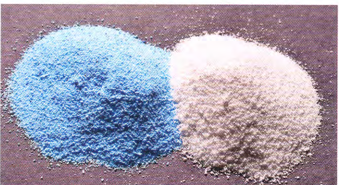
Webco's blended powders include some that are dyed for coloration. Materials discharged from the blender are thoroughly and uniformly mixed and ready for packaging.
